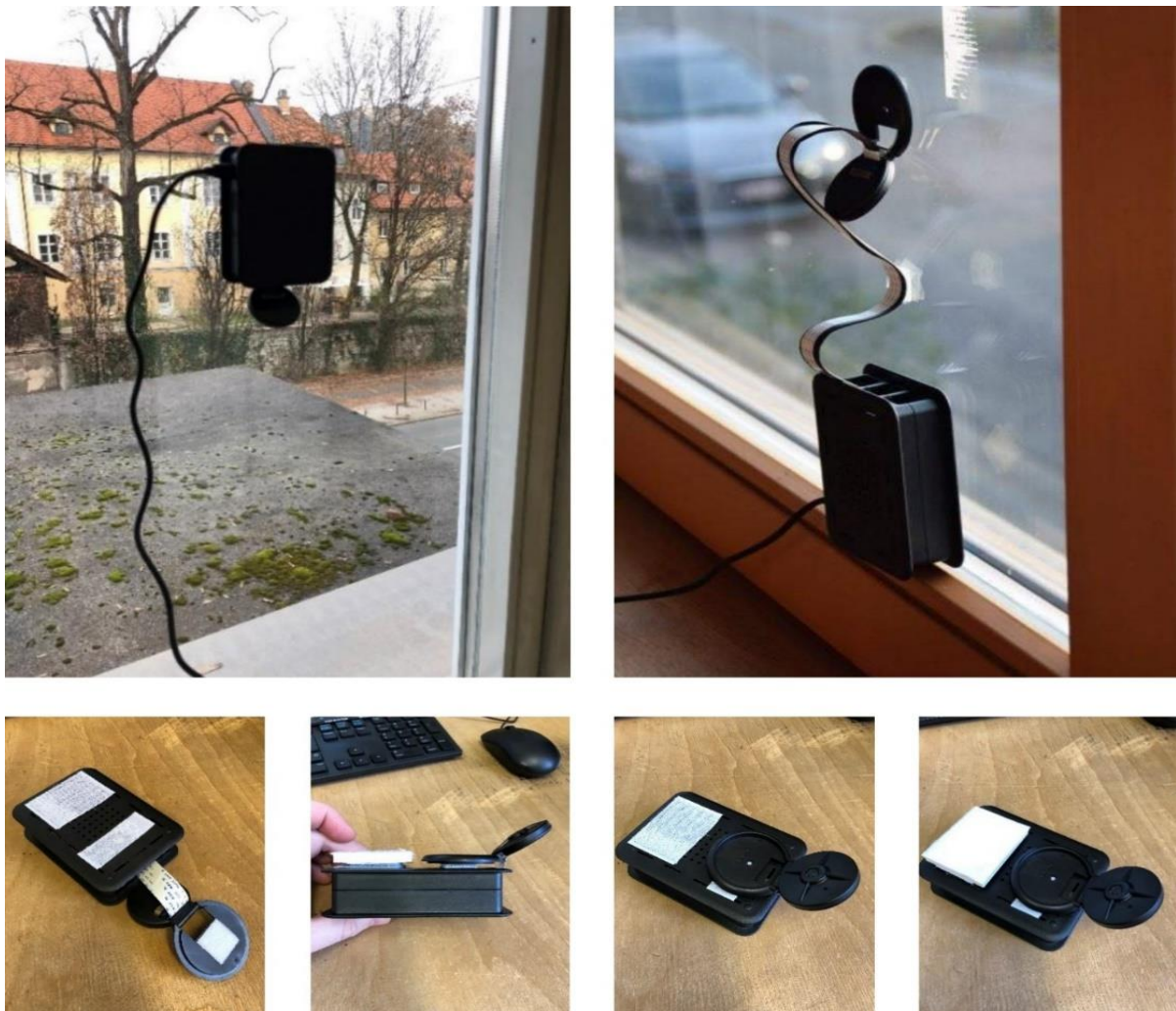
Figure 2: A simpler setup, shorter camera cables and eliminated need to apply black anti-reflective tape, thus avoiding reflections.
